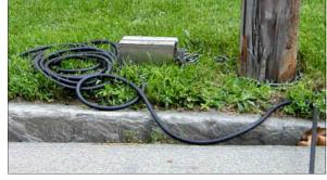
Traffic counters, like this one on East Seminary Ave. are being used throughout Vermilion County to determine traffic patterns. Data will be used to determine development and state- and federally-funded road repair projects.
